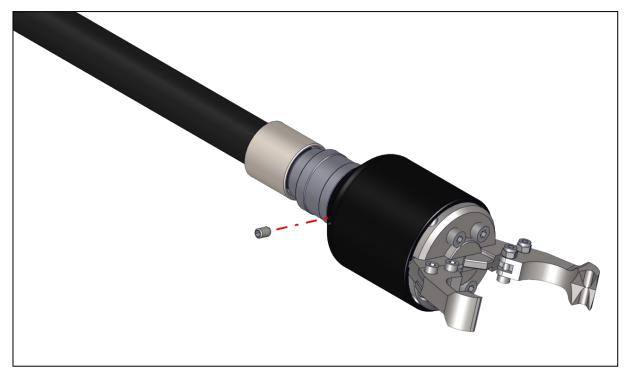
Step 2. Pull Cover aside and loosen four set screws attaching Grabber Head to the flexible shaft.
