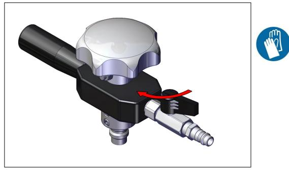
The Grabber can be rotated in the pipe by turning the knob handle which enables the user to turn the jaws to the correct position to grip the desired item. Rotate the knob handle only **clockwise**.
