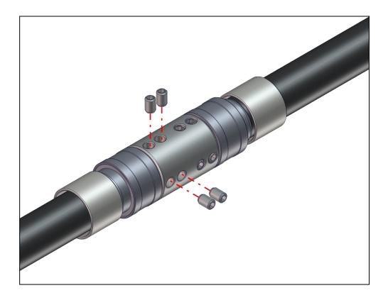
Step 9. Add the Control Head to the shaft again.
