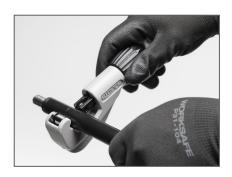
Always inspect the outer casing before each use. The easiest and safest way to shorten the outer casing to the correct length is using a sheath cutter. Only the necessary amount of bare shaft should be exposed at any time.
