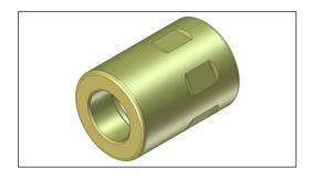
Always use a Sleeve when working with the Maxi Miller. It prolongs the lifetime of the flexible shaft and prevents the outer casing from melting in the tool end. The Sleeve can be reused when the outer casing has been shortened.
