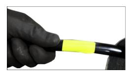
If not using a "leader" attach a visual marker (tape) on the outer casing of the flexible shaft. Place it around 500mm (20") from the end of the shaft. The marker will indicate the tools location and help prevent possible injury from the rotating parts by alerting you when the tool is about to exit the pipe.
