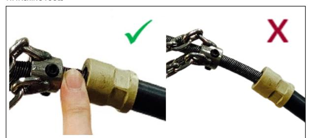
Keep the gap between the Sleeve Bearing and the Tool to 6mm (1/4")
