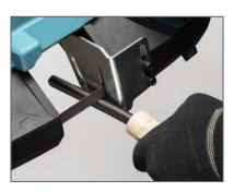
Always inspect the flexible shaft before each use. Run the machine briefly in clockwise direction to allow the shaft to return to it's resting position. If there are potential weak points or the shaft is damaged, cut off the damaged length using a band saw. For most tools, the shaft should extend ~40mm (1 ½") past the casing. Hubs and Original chains without a leader require more exposed shaft.
