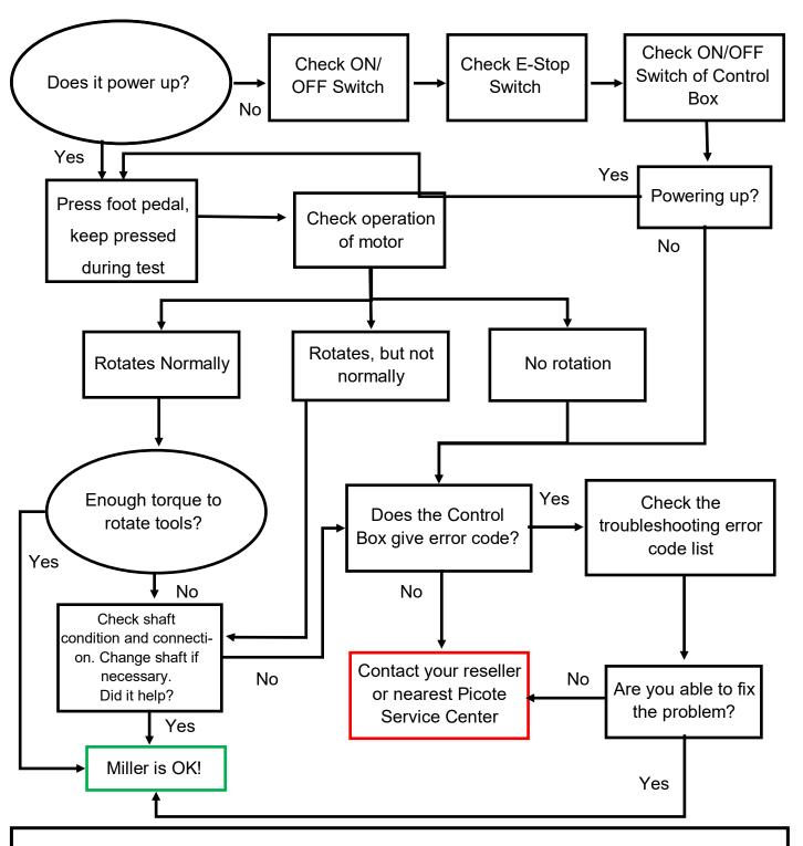
Write down the Error Code flashing in the screen of Control Box if needed to contact the Picote Service Centre. The Error Code narrows down the list of possible problems with your Miller unit.
