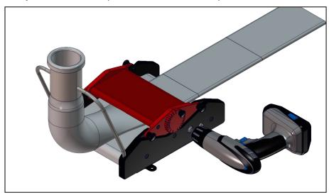
**Step 3.** Dispense the resin in accordance with the liner manufacturers instructions. To push the bulk resin through the Mini Roller, first open the two Index Plungers (showed below) and lift up the Upper Roller.
