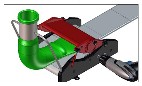
**Step 5.** Adjust the opening by turning the adjustment wheel if needed.
