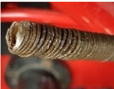
Damaged Shaft. Needs to be trimmed.
