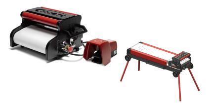
The new Hybrid Midi Roller is for wetting out CIPP liners from DN50-225 (2-9"). This lightweight and compact unit can be powered by the integrated battery or plugged in and charged during use.
