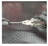
4. Use the tip of needle nosed pliers to slightly widen the end of the delivery hose.
